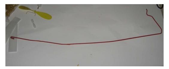
Insert the hook tool through the rocket body, and hook onto the rubber band motors.
