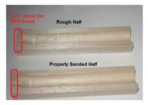
Second, do the two halves align properly? It's possible to have the outside edges of the wood match, but the inner holes not match. Hold your two halves together, and make sure the holes are aligned.
