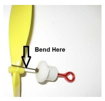
Install the Propeller onto the shaft.
