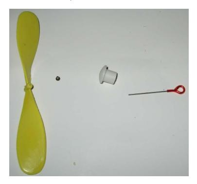
Insert the shaft through the nose piece, & bushing.
