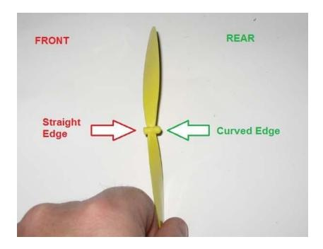
The propeller should have the rounded shaft-end pointing into (touching) the space derby (this makes the bending of the wire easier and it reduces friction). If you mix-up this assembly point, and install the straight edge facing the rocket body, your rocket will fly backwards!
