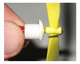
Install three rubber Band motors onto the shaft.
