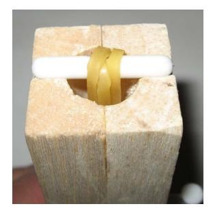
Do *not* glue the propeller assembly into the front of the space derby. It is pulled off to re-load new rubber bands!
